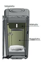
4. Remove the bottom stone by lifting it upwards and turning it to the side.
