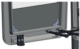
2. Remove the log guard, the grate and the ash pan.
