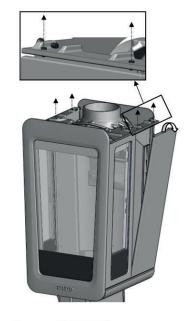
Please note that the lower part of the cast iron panel are located with two heels that fit into two holes in the stove body.
